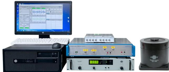
Accelerometer Calibration System SCS-ACV, according to ISO16063-21, is very suitable to middle-high frequency range (20Hz~5kHz). System include a vibration exciter BK4808, which is very suitable to small object. And force rating is 112N without cooling. The standard accelerometer Endevco 2270 is good at calibration application (Resonant Frequency $\geq$ 35kHz). System control and report generation are by software automatically.
