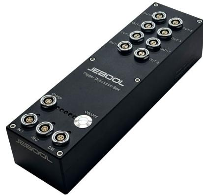
Trigger distributor box TRG-8S is mainly designed for vehicle crash test. It can also be used for multi-devices synchronous trigger during tests. The trigger input is usually connected to a ribbon switch or a photoelectric switch. Trigger outputs can connect with data acquisition, airbag squib device, cameras, etc. All channels are optically isolated. And built-in battery is with UPS function.
