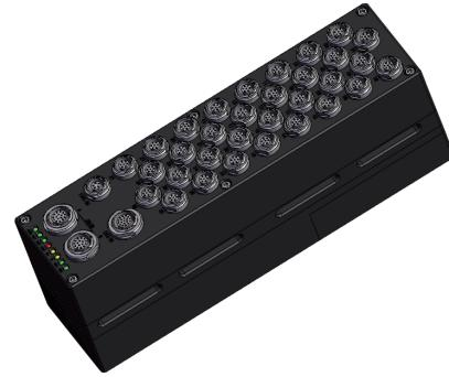
Onboard DAS JDAS-32C has an anti-shock design and very suitable to apply for crash test. The DAS support 32 channels sensor input (PR, SG Bridge, Pot. or Voltage) with excitation voltage and 16 channels digital input. A built-in UPS battery is used to ensure the reliability of communication and triggering. An independent trigger input can be connected to an external switch to realize start recording and T0 trigger mark.
