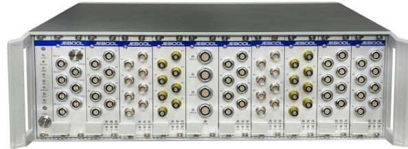
The JDAS-S adopts a modular expansion architecture, allowing flexible configuration of functional modules according to different testing needs, as well as future channel or module expansion. The basic chassis of the device includes power supply, status LED indicators, ethernet communication functions and trigger function. The system is operated with JEBOOL CrashPro software.
