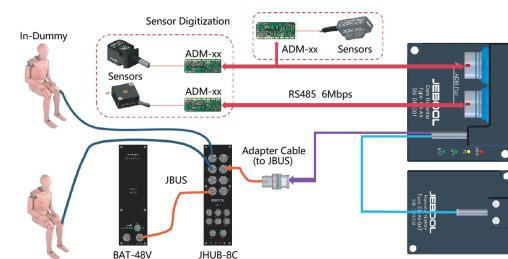
Note: DDAS is Digitization Data Acquisition System. It can record the sensor or signal data which converted by ADM modules.
