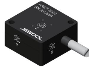
The 3-Axis angular rate sensor ARST-2002 is based on the principle of resonator gyroscope and contains multiple vibrating beams. When the structure rotation is detected, the capacity will be changed by Coriolis force generated. Then the angular rate can be measured by capacity converting into voltage signal. ARST-2002 supplies mounting positions for 3 pcs accelerometer 7264C. The length of wear-resistant cable and Dallas ID can be required.
