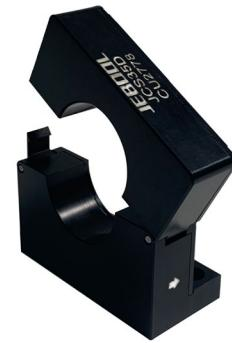
The current sensor JCS35D is based on the Hall principle to achieve high-precision measurement of line current. The independent power supply is completely isolated from the measurement system, and the direct output voltage signal has a good linear relationship with the measured current. JCS35D has default range 1000A, and below 2500A is optional.
