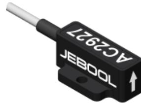
AC-100, based on MEMS, is a single axis accelerometer with very low noise. The sensor can real very high measurement repeatability. It includes an internal LDO to get stable accuracy voltage, which also reduces the sensor power supply. A RC decouple low pass filter is integrated to refine the signal output. The sensor includes wear-resisting cable with default length 8m. Also, the LEMO connector and Dallas ID are optional.
