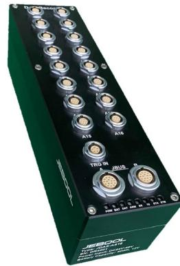
Onboard DAS JDAS-AS16 has an anti-shock design and very suitable to apply for crash test. The DAS support 16 channels sensor input (PR, SG Bridge, Pot. or Voltage) with excitation voltage. A built-in UPS battery is used to ensure the reliability of communication and triggering. An independent trigger input can be connected to an external switch to realize start recording and T0 trigger mark.
