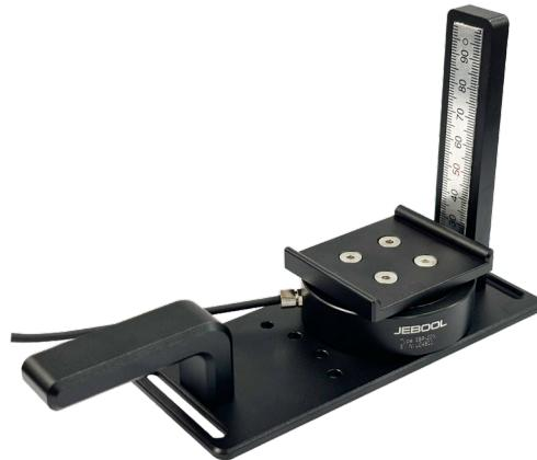
The seatbelt press force sensor includes a high-precision sensor unit combined with fixture, making it convenient to measure press force by seat belts on dummy. The fixture has a height gauge, and easy to measure the seatbelt lifting height. During testing, the components can be disassembled as needed, retaining only the necessary parts to meet specific application requirements.
