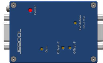
The signal conditioner BR-SC1A is used in the precise amplification of millivolt or microvolt voltage signals, while maintaining a high signal transmission bandwidth. For strain gauge bridges and piezoresistive type sensors, a precision excitation voltage with compensation is provided. At the same time, BR-SC1A has a built-in power filter module, which effectively suppresses the interference when the external power supply is with noise.
