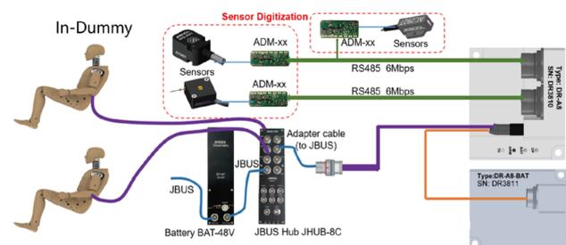
Note: DDAS is Digitization Data Acquisition System. It can record the sensor or signal data which converted by ADM modules.
