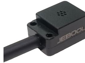
Pressure sensor DP200K, based on piezo resistance effect, zero at ambient, includes a full bridge circuit. There is resistance changed by measuring different air pressure, then the voltage signal can be converted according to the resistance difference. The reasonable MEMS process makes the sensor good linearity performance and stability. The sensor includes wear-resisting cable with default length 8m. The LEMO connector and Dallas ID are optional.
