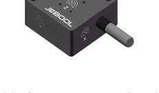
The 3-Axis angular rate sensor ARST-2002 is based on the principle of resonator gyroscope and contains multiple vibrating beams. When the structure rotation is detected, the capacity will be changed by Coriolis force generated. Then the angular rate can be measured by capacity converting into voltage signal. ARST-2002 supplies mounting positions for 3 pcs accelerometer 7264C. The length of wear-resistant cable and Dallas ID can be required.
