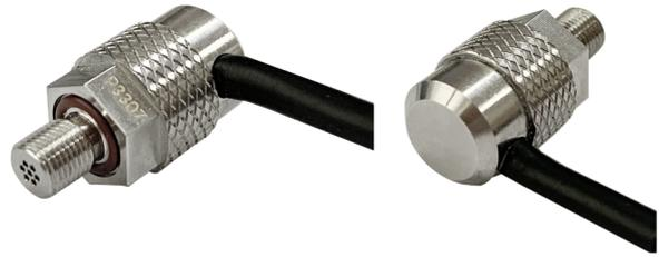
Pressure sensor AP50KL, based on piezo resistance effect, zero at ambient, includes a full bridge circuit. There is resistance changed by measuring different air pressure, then the voltage signal can be converted according to the resistance difference. The reasonable MEMS process makes the sensor good linearity performance and stability. The sensor includes wear-resisting cable with default length 8m. The LEMO connector and Dallas ID are optional.
