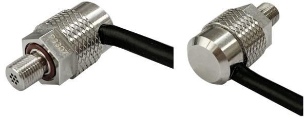
Pressure sensor AP200KL, based on piezo resistance effect, zero at ambient, includes a full bridge circuit. There is resistance changed by measuring different air pressure, then the voltage signal can be converted according to the resistance difference. The reasonable MEMS process makes the sensor good linearity performance and stability. The sensor includes wear-resisting cable with default length 8m. The LEMO connector and Dallas ID are optional.
