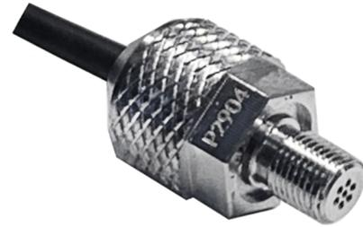
Pressure sensor AP500K, based on piezo resistance effect, zero at ambient, includes a full bridge circuit. There is resistance changed by measuring different air pressure, then the voltage signal can be converted according to the resistance difference. The reasonable MEMS process makes the sensor good linearity performance and stability. The sensor includes wear-resisting cable with default length 8m. The LEMO connector and Dallas ID are optional.
