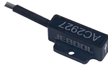
AC-200, based on MEMS, is a single axis accelerometer with very low noise. The sensor can real very high measurement repeatability. It includes an internal LDO to get stable accuracy voltage, which also reduces the sensor power supply. A RC decouple low pass filter is integrated to refine the signal output. The sensor includes wear-resisting cable with default length 8m. Also, the LEMO connector and Dallas ID are optional.
