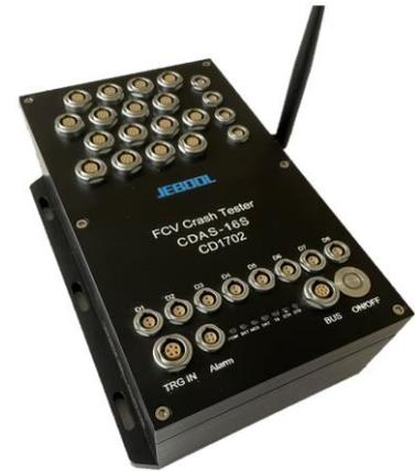
CDAS-16S is designed for HFCV leak measurement during crash tests according to ECE R13. The data can be display on the PC by WiFi and storage internal at the same time. It is very suitable to monitor the FCV SAFETY post-crash. The sensor SM-05D and H2-5B (He-5B) can be connected to measure containers valve status and gas concentration percent in the air. The cables that pressure and temperature signals input into device could be supplied, based on the connector types of sensors.
