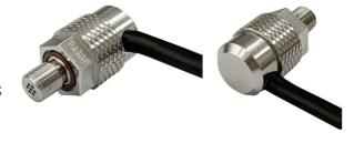
Pressure sensor AP200KL, based on piezo resistance effect, zero at ambient, includes a full bridge circuit. There is resistance changed by measuring different air pressure, then the voltage signal can be converted according to the resistance difference. The reasonable MEMS process makes the sensor good linearity performance and stability. The sensor includes wear-resisting cable with default length 8m. The LEMO connector and Dallas ID are optional.
