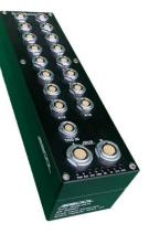
Onboard DAS JDAS-AS16 has an anti-shock design and very suitable to apply for crash test. The DAS support 16 channels sensor input (PR, SG Bridge, Pot. or Voltage) with excitation voltage. A built-in UPS battery is used to ensure the reliability of communication and triggering. An independent trigger input can be connected to an external switch to realize start recording and T0 trigger mark.
