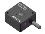
The 3-Axis angular rate sensor ARST-2002 is based on the principle of resonator gyroscope and contains multiple vibrating beams. When the structure rotation is detected, the capacity will be changed by Coriolis force generated. Then the angular rate can be measured by capacity converting into voltage signal. ARST-2002 supplies mounting positions for 3 pcs accelerometer 7264C. The length of wear-resistant cable and Dallas ID can be required.
