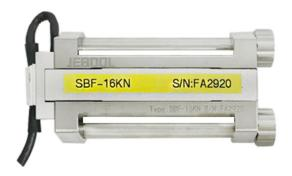
Seatbelt force sensor based on full bridge takes the principle of strain and transfers the internal tension of the belt to sensor structure. The strain structure can change resistance different, and then convert it into voltage change. The main structure of sensor is made of titanium alloy material to reduce its weight to other effects. SBF-16kN is equipped with high performance wear cable. Dallas ID and the connector depend on customers.
