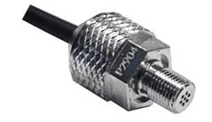
Pressure sensor AP1000K, based on piezo resistance effect, zero at ambient, includes a full bridge circuit. There is resistance changed by measuring different air pressure, then the voltage signal can be converted according to the resistance difference. The reasonable MEMS process makes the sensor good linearity performance and stability. The sensor includes wear-resisting cable with default length 8m. The LEMO connector and Dallas ID are optional.
