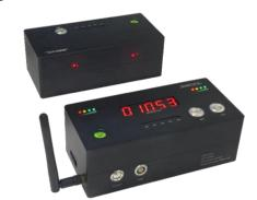
Speed Measurement Device SPS-5M, by two groups of high-speed laser sensors of front and rear installed in opposite direction, can detect the time difference of the object passing through the two sets of laser sensors. So that the speed can be calculated because the length is constant. The result can display by internal LED or external LED, and even remote PC.
